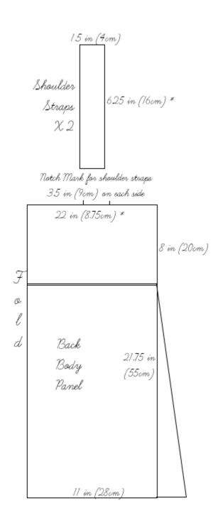
3. The diagram shows the pattern for a size 4-6 (UK size 8-10). Adjust by adding 1 inch (2.5cm) to each seam for each size up, or take away an inch
